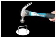
Tip: Tap threaded retainer ring to loosen dirt and silt before turning the ring counter-clockwise.
