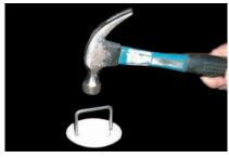
Tip: Tap threaded retainer ring to loosen dirt and silt before turning the ring counter-clockwise.
